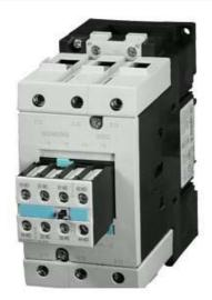
CONTACTOR, AC-3 30 KW/400 V, AC 220V 50HZ/240V 60HZ 2 NO + 2 NC 3-POLE, SIZE S3, SCREW CONNECTION
